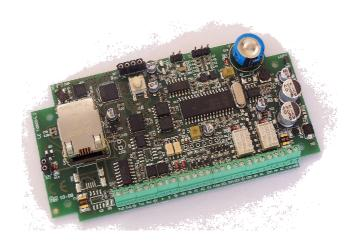
The **IDSOFT OEM** is an Embedded RFID board for both 125KHz and 13.56MHz frequencies.
